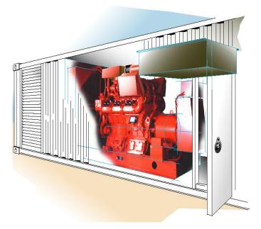
The ICHM is connected to the IC engine generator coolant loop and to the building hydronic loops. The unit is driven with the heat rejected by the engine and provides both cooling and heating. The cooling and heating heat exchangers are in series and normally operate simultaneously for high load factor. Condenser water will be provided by the buildings main cooling tower loop.
